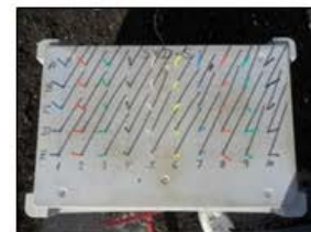
Manifold for sampling one transects 50 gas probes
