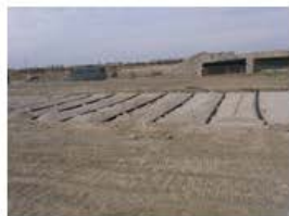
GDL with pipes and zig-zag shaped interface
