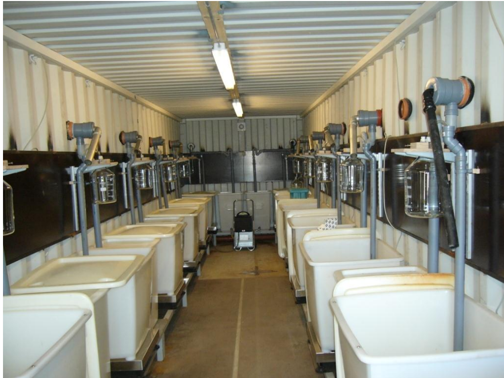
2.10 View of the leachate collection and sampling systems in the shipping container.
