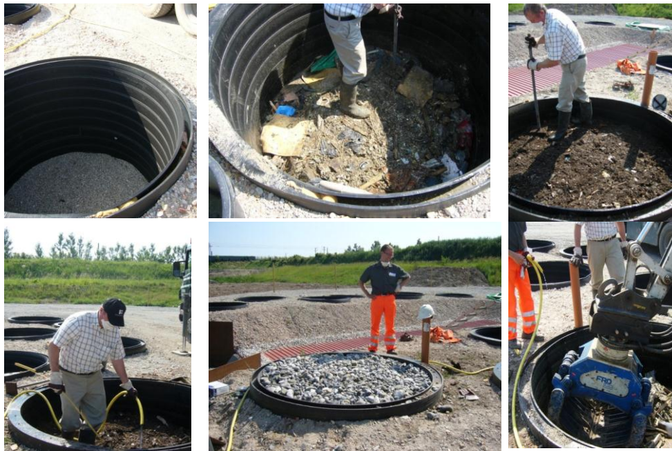
Figure 2.12 Pictures of the filling of the lysimeters on 7 June 2007.
