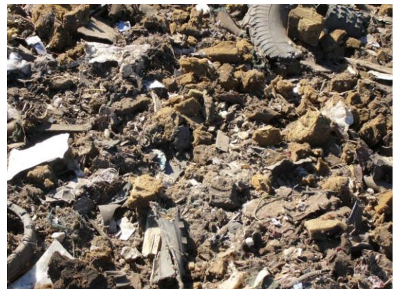
Figure 2.2 Surface of shredder waste in landfill.
